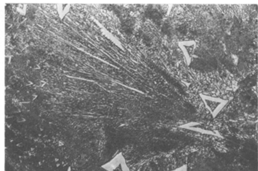
Figure 7 Microstructure of a 95 mol% \text{GeO}_2 composition showing crystallization of primary \text{BaGe}_4\text{O}_9 in a eutectic matrix containing \text{BaGe}_4\text{O}_9 and \text{GeO}_2 ( \times 250 ).
