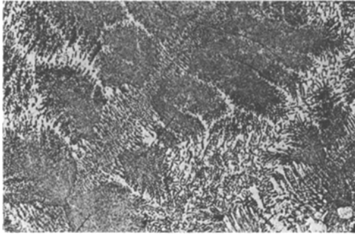
Figure 5 Microstructure of a 61.5 mol% \text{GeO}_2 composition exhibiting a complete eutectic structure between \text{BaGeO}_3 and \text{BaGe}_4\text{O}_9 ( \times 200 ).
